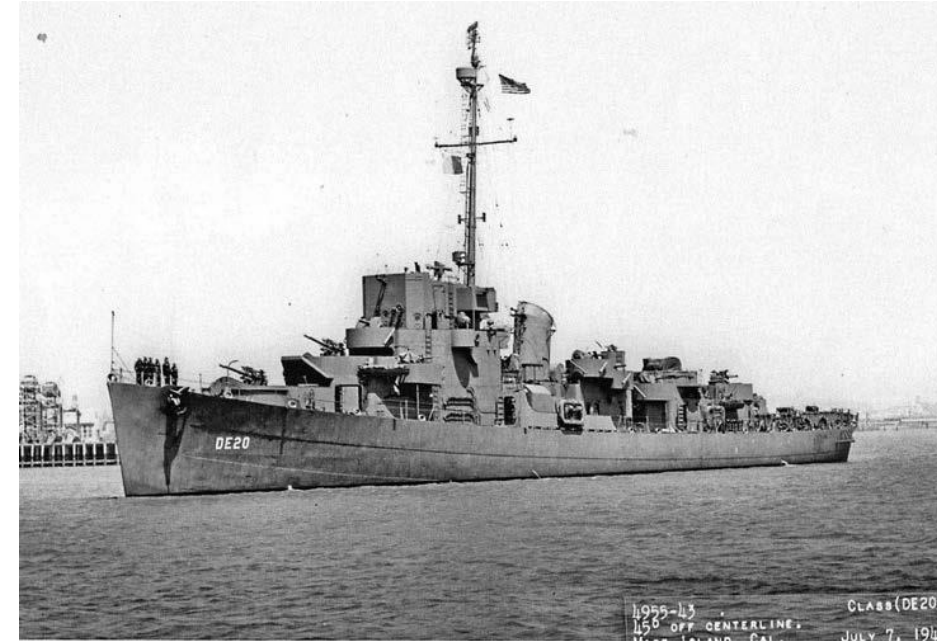
USS LeHardy (DE 20) in the Mare Island Channel, 1943. ( http://www.navsourc.org/archives/06/images/020/0602016.jpg accessed 28 May 2018). This ship is of the Evarts class, which was fitted with diesel-electric drive of half the originally designed shaft horsepower (Silverstone 1965).
